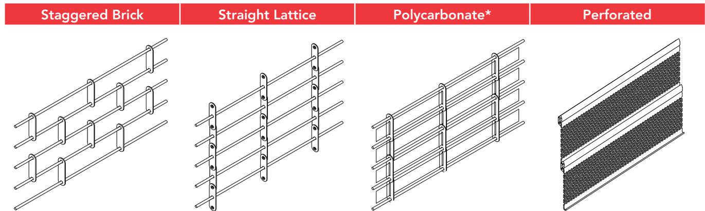
Note: These products allow air infiltration and are not weather tight.
